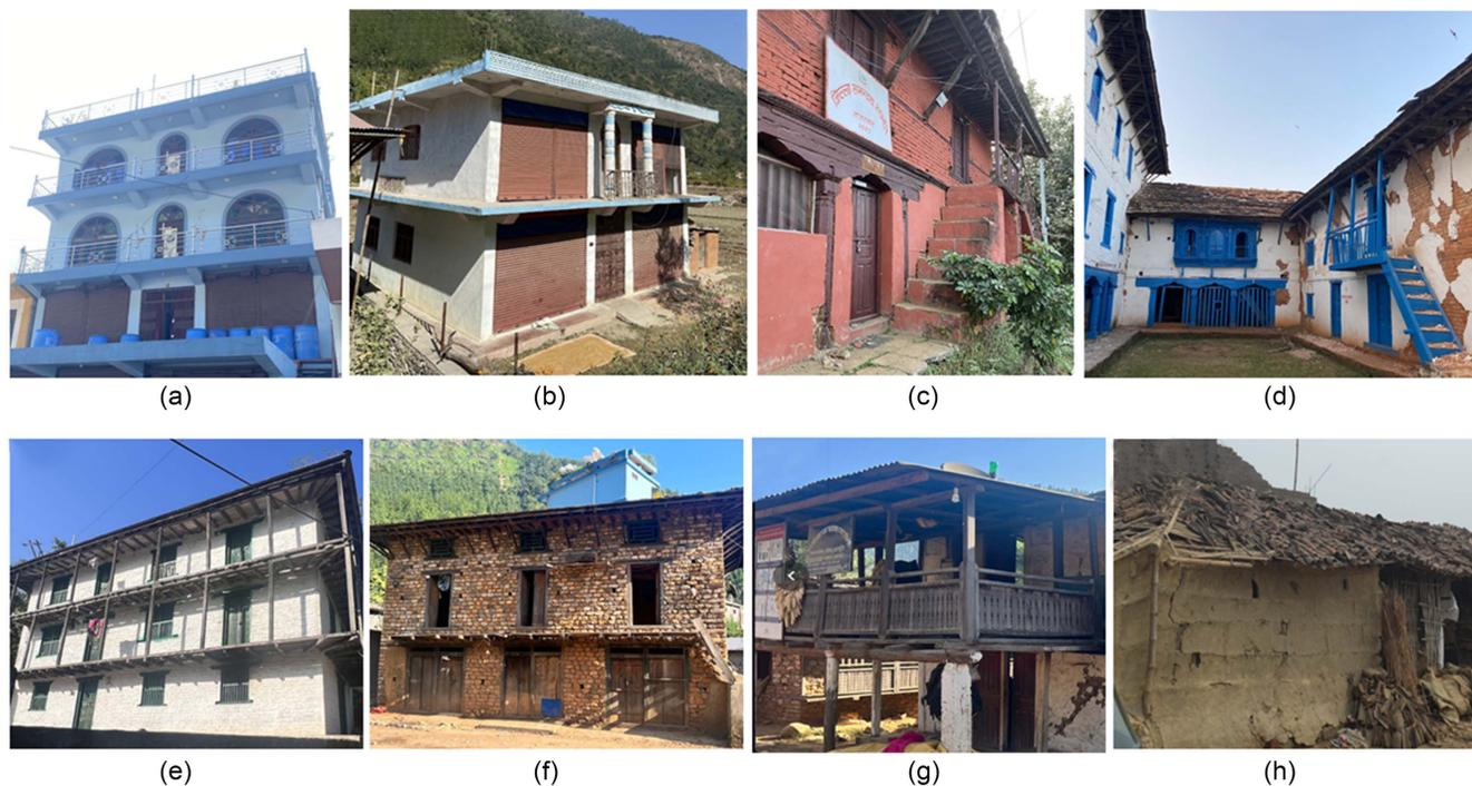
**Fig. 2.** Existing building types in Nepal: (a) engineered RC; (b) nonengineered RC; (c) brick in cement mortar; (d) brick in mud mortar; (e) stone in cement mortar; (f) stone in mud mortar; (g) wooden; and (h) adobe. (Images by Rajan KC.)
