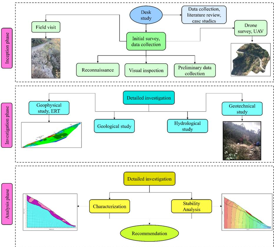
Fig. 2 Flowchart of detailed methodology of the slope stability study
