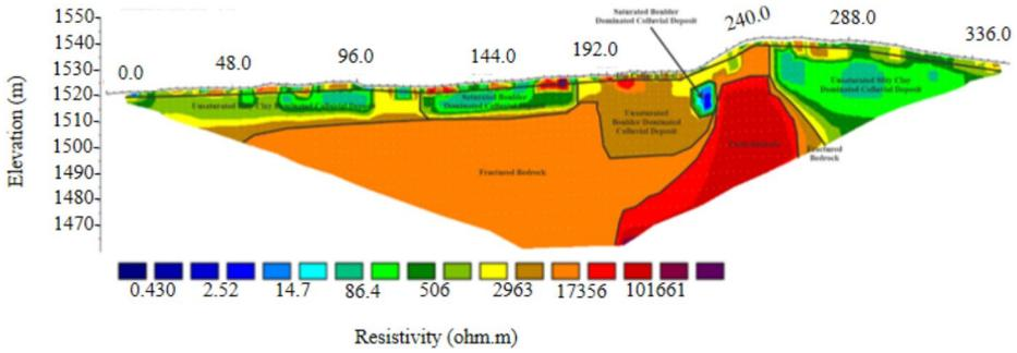
**Fig. 6** ERT-1 profile inversion result and interpreted lithology showing different soil layers: colluvial deposits overlying the fractured bedrock
