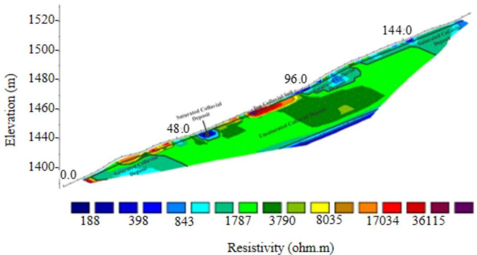
**Fig. 7** ERT-2 profile inversion result and interpreted lithology showing different soil layers: colluvial deposits overlying the saturated fractured bedrock
