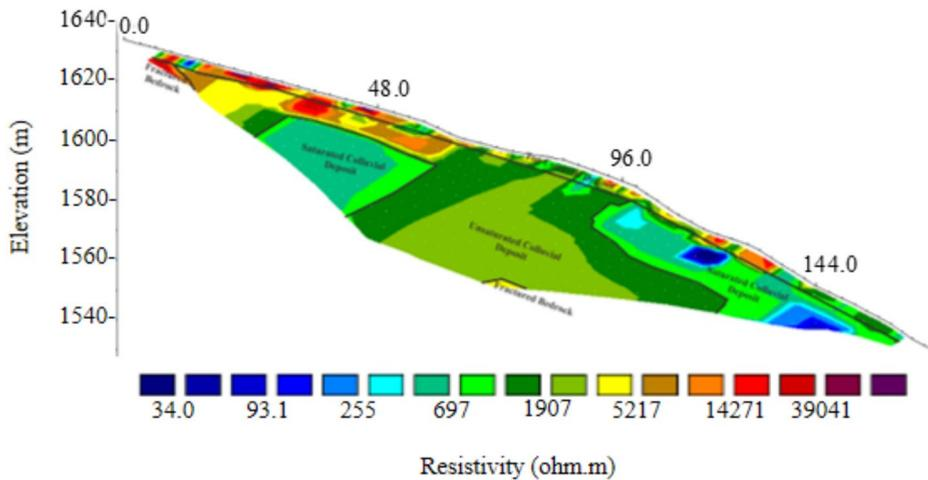
**Fig. 8** ERT-3 profile inversion result and interpreted lithology showing different soil layers: saturated and unsaturated colluvial deposits
