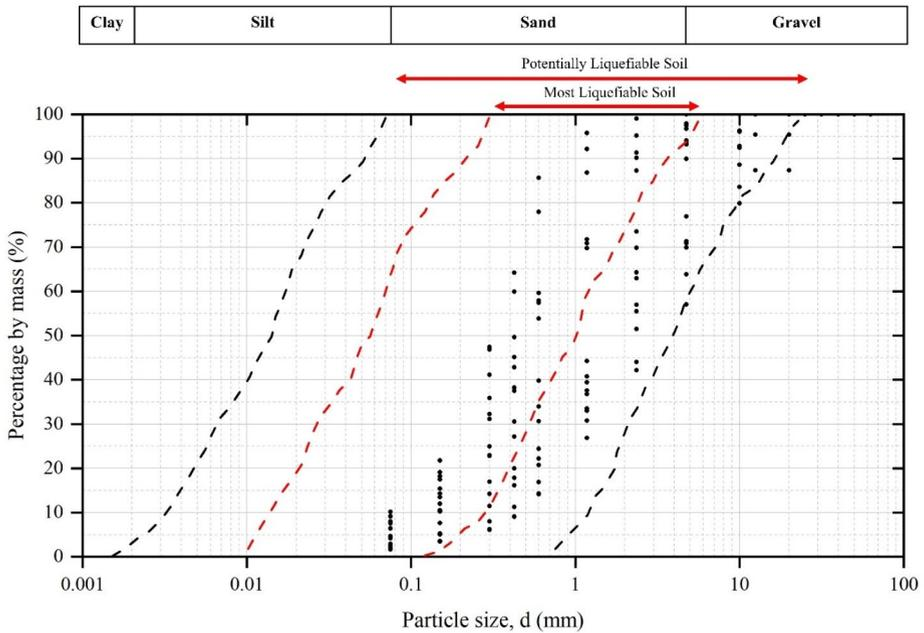
**Fig. 10** Particle size distribution graph of the site soils from BH-1 and BH-2 at different depths with a demarcation of liquefiable soils suggested by Tsuchida and Hayashi (1972)
