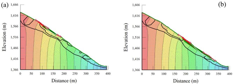
**Fig. 12** SLOPE/W Output under existing conditions: (a) SLOPE/W output indicating possible slip surface on hillside with FOS=0.791, (b) SLOPE/W output indicating possible slip surface on valley side with FOS=0.799
