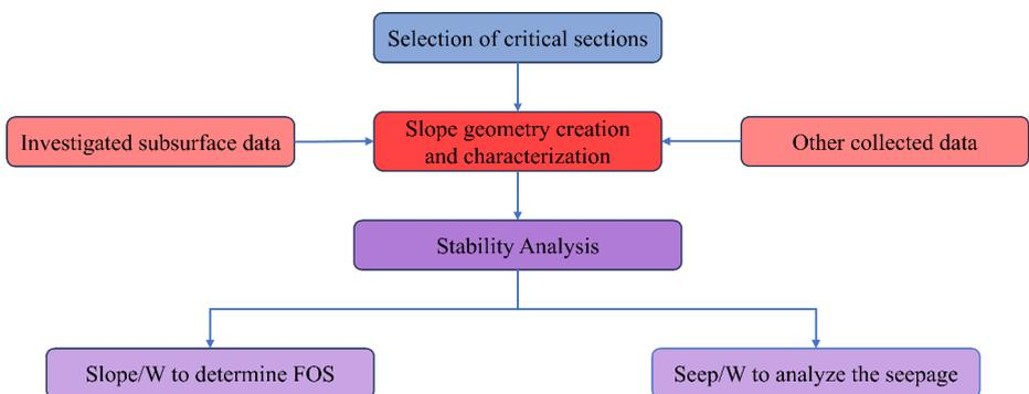
**Fig. 5** Flowchart illustrating the steps involved in the analysis of slope stability using GEOSTUDIO
