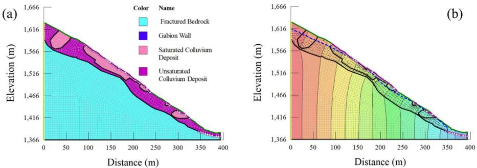
**Fig. 11** (a) Interpreted GEOSTUDIO model of the critical section, (b) SEEP/W output under existing condition showing Seepage pockets and groundwater level
