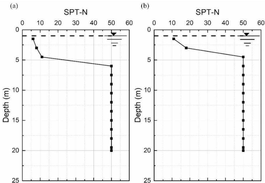
Fig. 9 Borehole logs showing SPT N-values and groundwater level of (a) BH-1 and (b) BH-2
